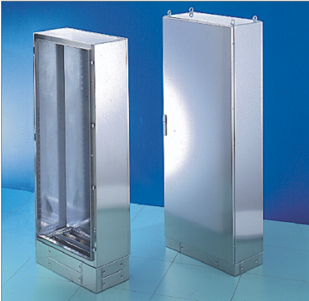
"TFR" - "TFR/V" Modular stainless steel Aisi 304, cabinets with closed sides, complete with reversible solid or transparent door/s, removable rear panel, removable bottom plates with flanges for cable entry. IP55 protection.
