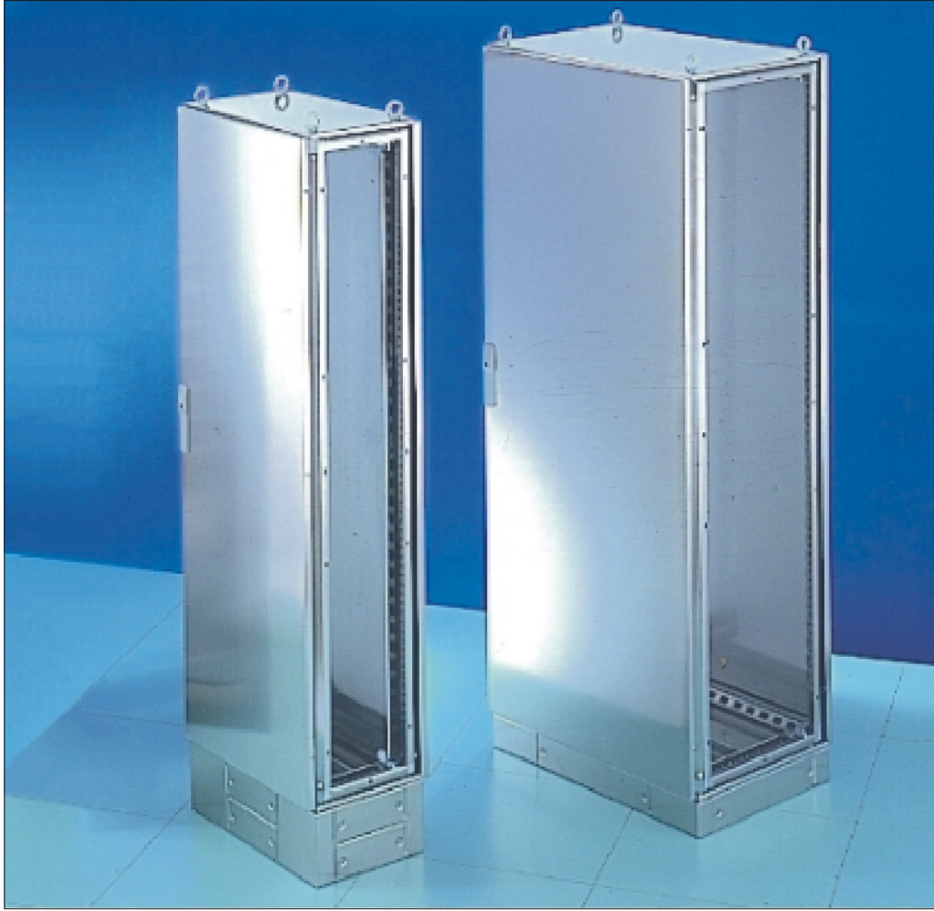
"TSR" - "TSR/V" Modular stainless steel Aisi 304, cabinets complete with reversible solid or transparent door/s, removable rear panel, removable top, removable bottom plates with flanges for cable entry. IP55 protection.
